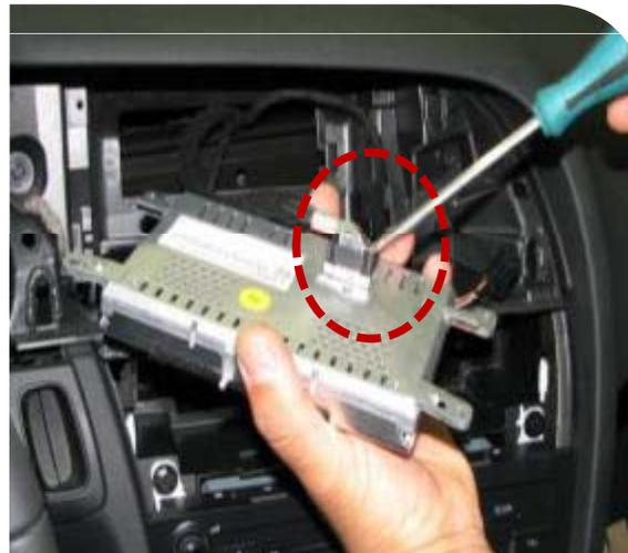
Remove the screws with a proper tool and monitor like the left picture.
