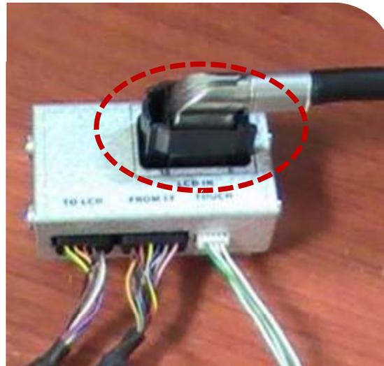
Connect the original LCD cable from monitor to "LCD-IN" of provided sub-board.
