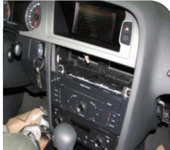
Remove the Air-Con. Box with proper tools as the left picture.
