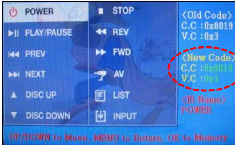
3. As soon as pressing the button, the remote button value displays at the right corner and it is saved automatically.
