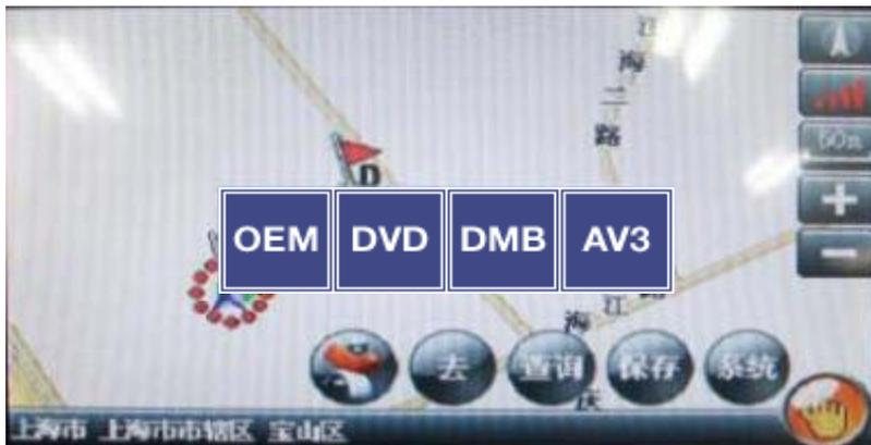
When Navigation is operated, if touching any point at the screen for more than 2 sec, Mode change menu will be appeared at the middle of the screen like left picture, navigation will stop temporarily and once touching any point excluding "menu" at the screen, it gets back to operation.
