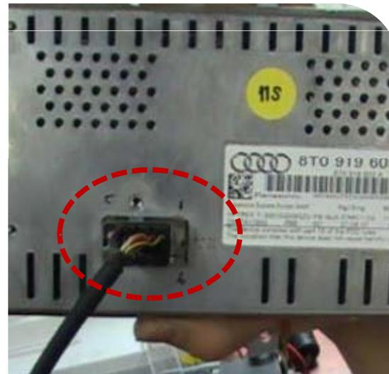
Connect the provided LCD-OUT cable between behind of LCD monitor and provided sub-board like left pictures.
