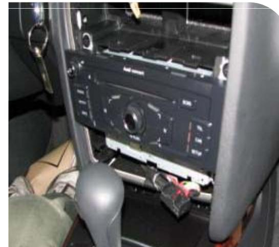
Remove the indicated part under the head unit with proper tools like the picture.
