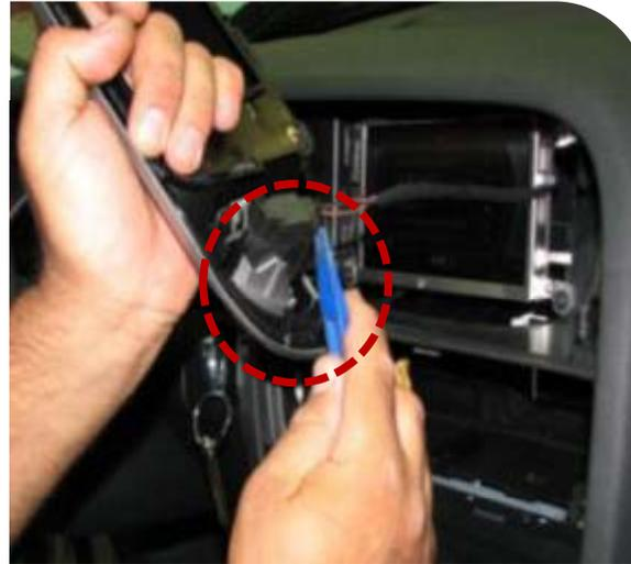
Remove the LCD case with a proper tool, be careful of the cable connected with the case.
