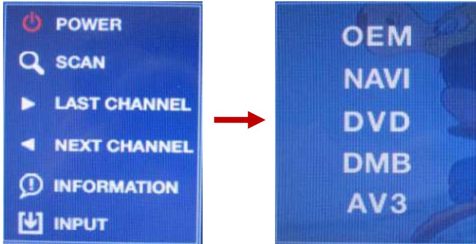
On AV2 mode, once touch the screen, Menu window appears like left picture. If no action for 5 sec or touch any other parts of the screen, this will disappear.
