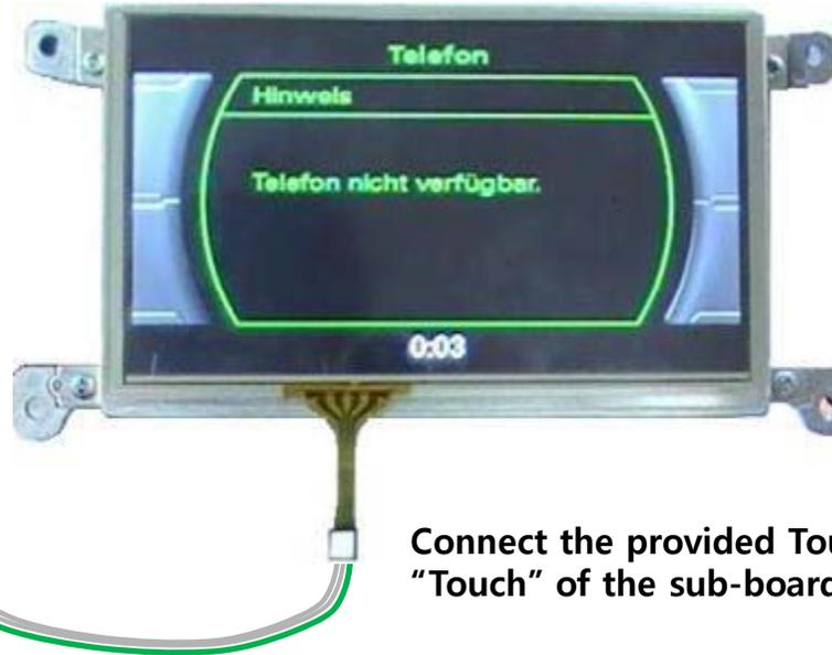
Connect the provided Touch Screen Cable to "Touch" of the sub-board and Touch Screen.
