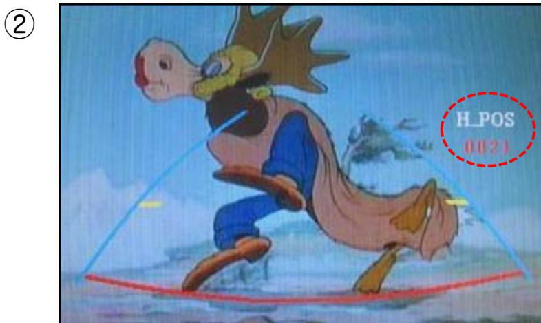
② After the setting done, rear parking guide line will appear in rear gear position. Once press "OK" button, "H\_POS" appears at the right and can adjust the line's position.
