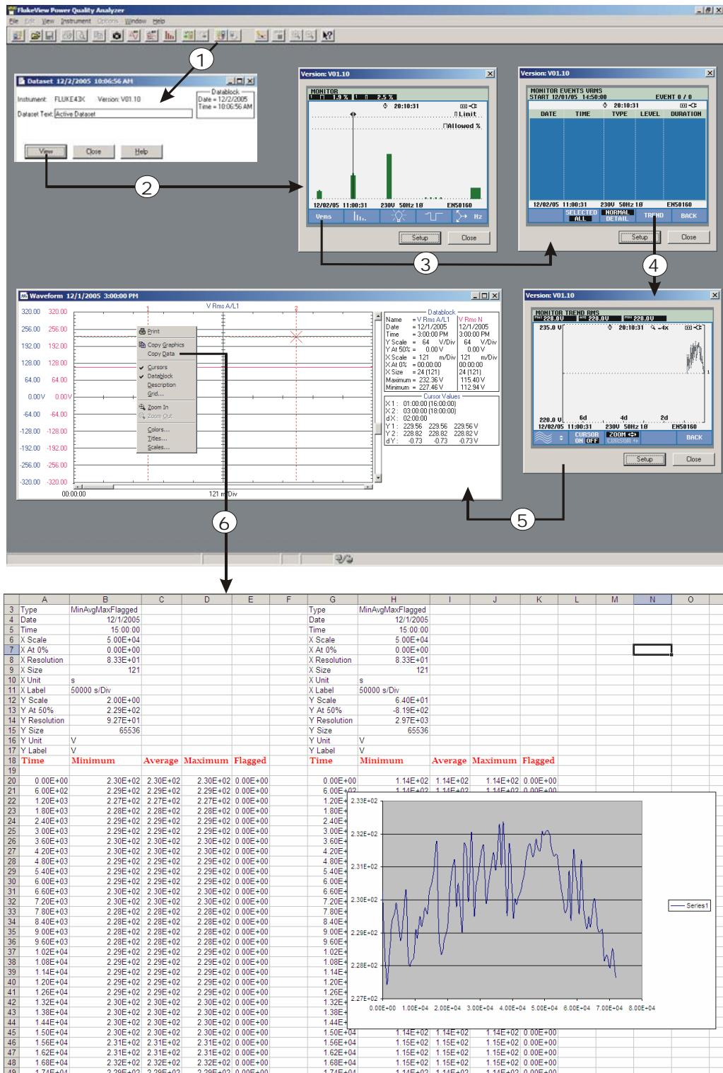
In this example column A (time axis) and column B (Min. Voltage trend 1) are graphed using the Excel Chart Wizard.
